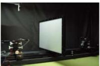
The tested light is installed to face the CCD camera with a standard diffusion plate attached at the position of the working distance at which the measurement is performed. A lens that can cover the whole illumination pattern is attached, and the measurement conducted. The results are uploaded to a computer to obtain the data on 2D luminance level distribution and luminance level variation on the X and Y axes. Measurement data can also be produced using an illuminometer upon request.
