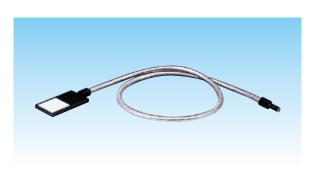
These plate type light guides do not require much space due to their slim, compact design. Moritex's unique reflected light inducer allows for even and bright illumination. They can be used for multi-observation inspections that require transmitted and uniform illumination such as backlighting electronic components or semi-transparent surfaces.
